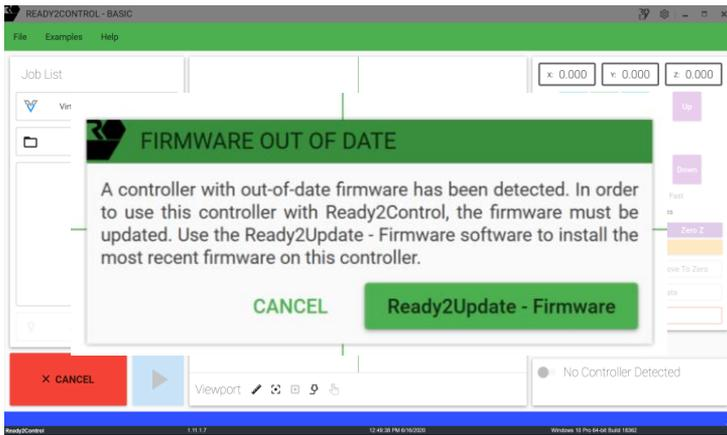
**3.2** The **FIRMWARE OUT OF DATE** pop-up window may appear the first time you connect Ready2Control to your Next Wave CNC machine. Click the **Ready2Update-Firmware** button to start the update process.
