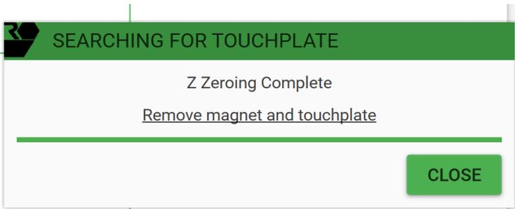
**Step 6** Remove the magnet and touchplate from the machine before proceeding.
